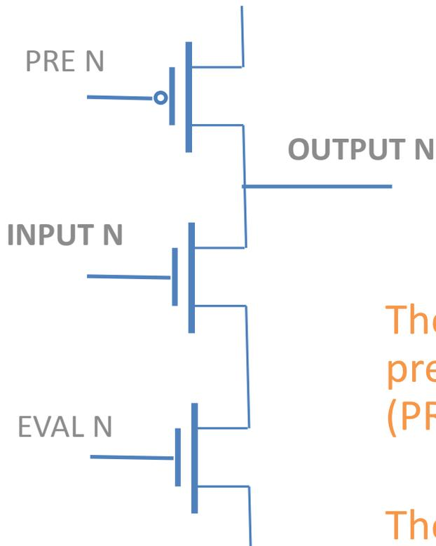
The inverter needs a precharge signal (PRE) to be activated.
