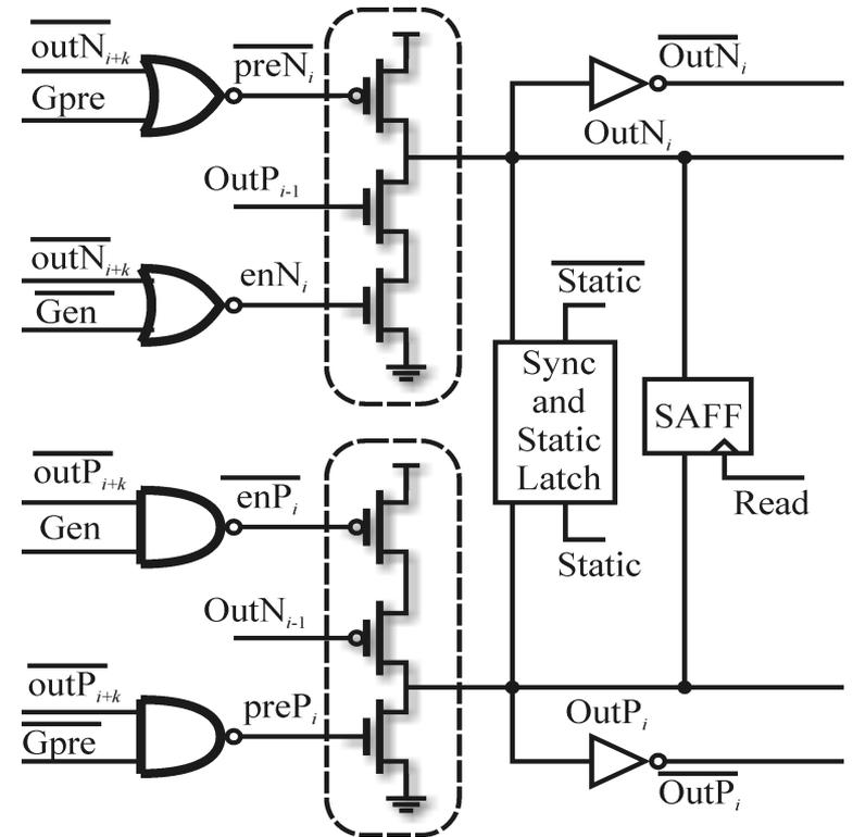
The output is stabilized by the latch and acquired by a Strong Arm FF
