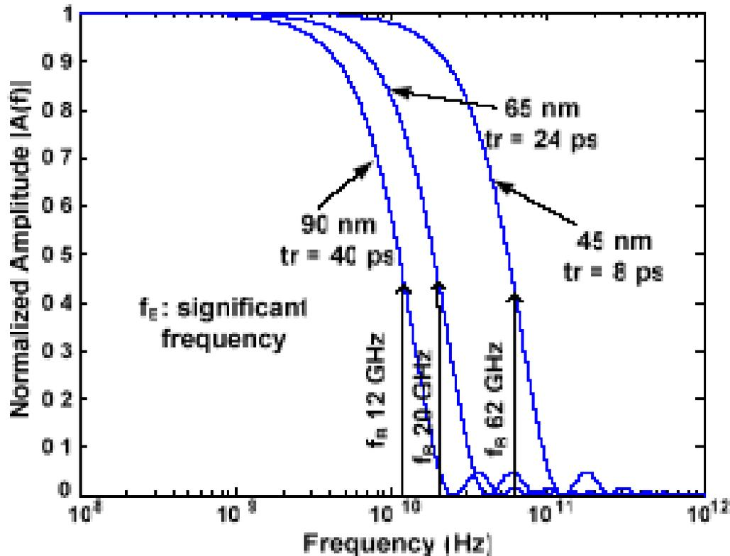
**CMOS bandwidths from 90 to 45 nm technology nodes (ITRS 2005)**
