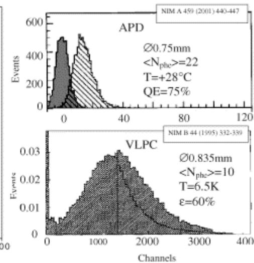
Fig. 3. SiPM application for sci fiber MIP detection (at room temperature): comparison with APD [6] (room temperature) and VLPC [7] (6.5°K).
