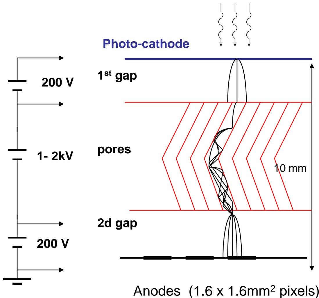
Pore diameter: a few  $\mu\text{m}$
