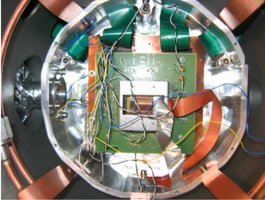
Figure 19: Inner view of the IR bench cryostat showing the ASIC on its electronic card surrounded by the thermal screen.
