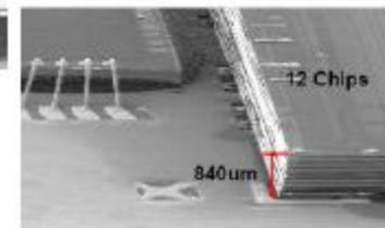
Samsung - 30 um laser drilled vias in 70um chips
