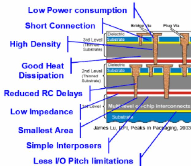
TSV interconnects provide solutions to many limitations of current SiP and Chip Stacking methods.
