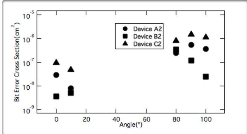
Bit Error Cross Section as a function of the incidence angle,
