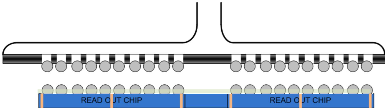
Solder mass transfer is very efficient process to attach the solder spheres to wafer
